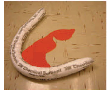
Use the mini-boom to block the spill from spreading under furniture or into floor drains.
